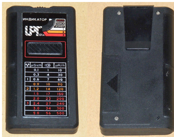
Fot. 6. Indykator promieniowania gamma IRG-01A Photo 6. IRG-01A gamma radiation indicator
